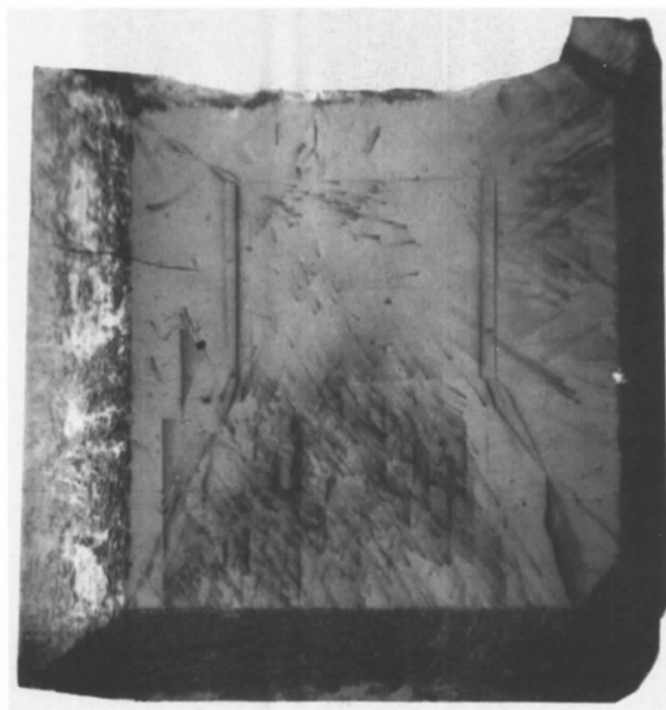
Fig. 4. The 311 \text{Cu } K\alpha_1 single-crystal back-reflection projection topograph, presenting the configuration of stacking faults close to the investigated surface of the slab cut from the De Beers synthetic octahedral diamond. The plane of diffraction is located horizontally.
